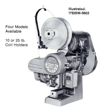
115 VAC, 60 cycle Single Phase 1/4 hp Motor. 1140 rpm with low voltage protection and push button start-stop switch, with relay. Solenoid-Operated Clutch with all foot and finger guards.
